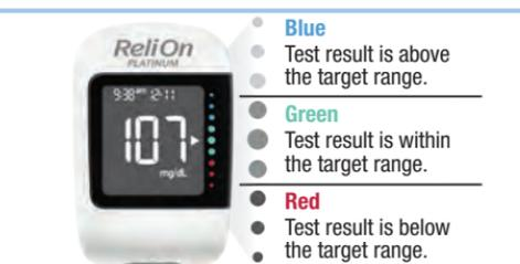
Your test result appears with an arrow. This arrow shows if your test result falls above, within, or below the target range.\* The target range is represented by the green region of the target range indicator. The arrow will flash if your test result falls above or below this range.
