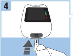
Insert the metallic end of the test strip into the meter.
